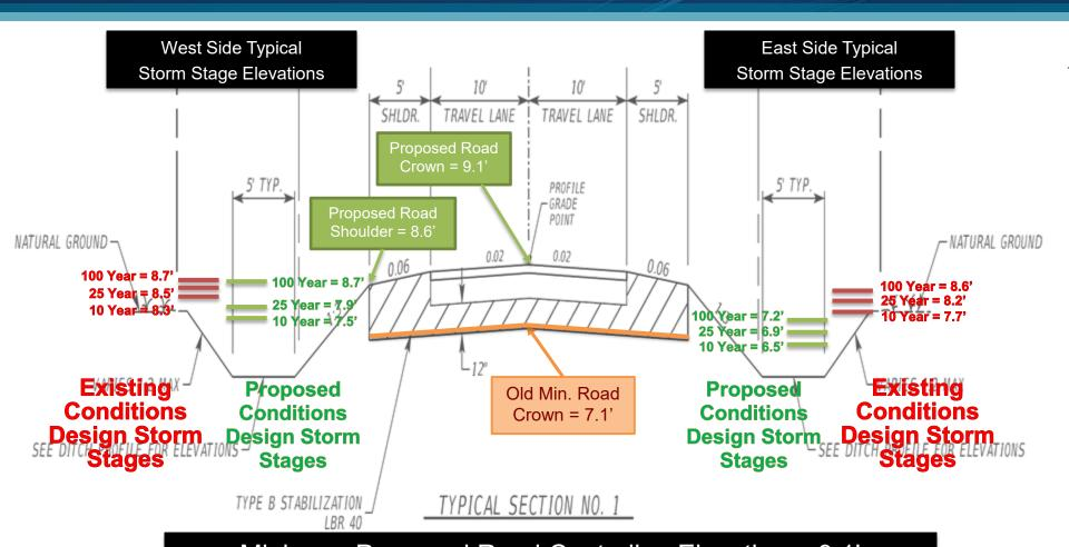
Minimum Proposed Road Centerline Elevation = 9.1'
